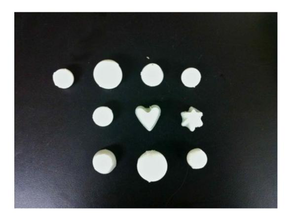
After the implants are ready, make the gel with the appropriate PVA concentration for the main brain. Put the implants inside and fill the brain mold with the gel. To save your time and material, it is suggested to fill the mold with water first, and measure the volume of the water to know how much PVA you will need to make the phantom. However, if you don't want to wet your mold, some couscous will work the same.
