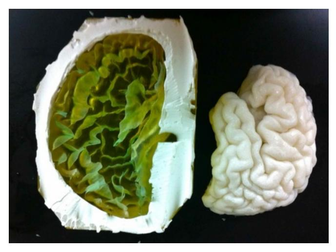
The most difficulty I had with the cooking is really dissolving the PVA crystals into water. To melt the crystals while not burning them into some yellow colour, you should prepare your water to be between 70 ~90 degrees Celsius, and keep stirring. In this sense, a nice water bath and a thermometer will be very instrumental. Also, watch out for the loss of H2O through the cooking process. Too much water loss may mean that your concentration will go up, resulting in a harder material.
